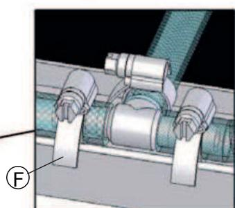
Reducire le tuyau au minimum / Reduce the pipe to the smaller size /
